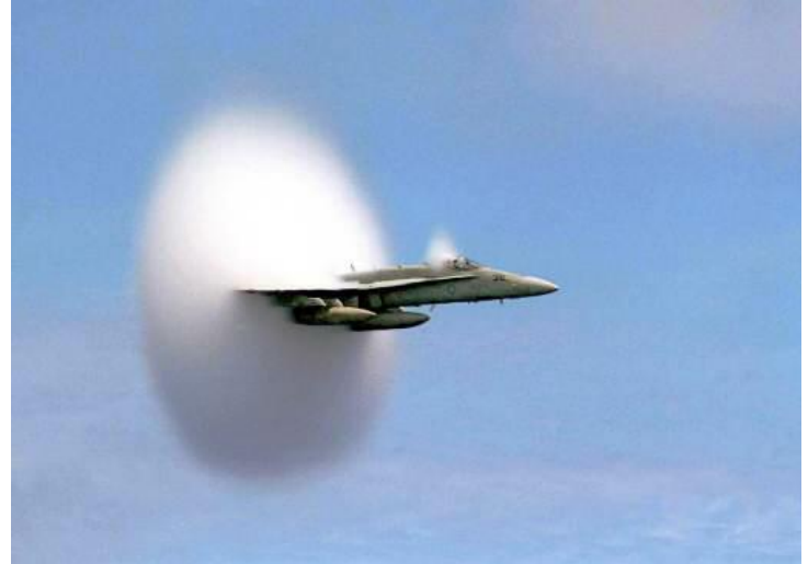
Condensation cloud as an F/A-18 Hornet flies at or near the speed of sound. Photo by John Gay.
